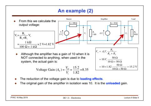
If the amplifier were ideal, since its voltage gain is x10, we would expect the output to be 20V.
