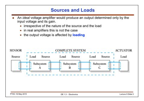
In electronic systems, there can be a number of amplification stages connected in series (also known as cascade). In the system shown here, a sensor may produce the **source** of the electrical signal. This could be passed through three stages to drive an actuator, which is the final **load**.
