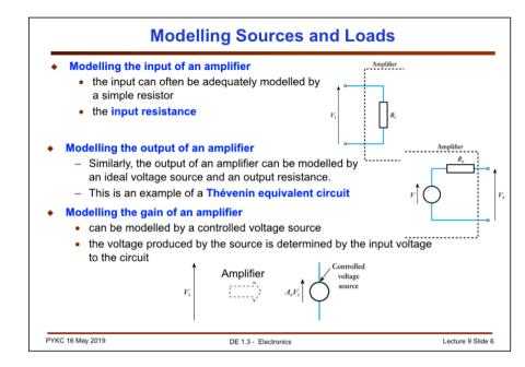
Consider an actual input of an amplifier. Its input can be modelled as an **input resistance**  $R_i$  as shown in the figure here. In an ideal amplifier,  $R_i = \infty$ . In real amplifier  $R_i$  is large but finite.
