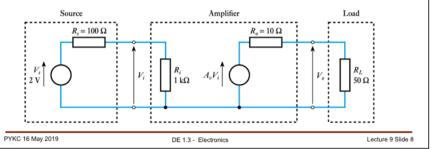
Let us now consider an example. We assume that source voltage is a 2V battery with a  $100\Omega$  source resistance  $R_S.$  This source signal is applied to the input of an amplifier  $V_I$  with a  $1k\Omega$  input resistance, a gain of 10 and a  $10\Omega$  output resistance. The output of the amplifier  $V_O$  is driving a  $50\Omega$  load.
